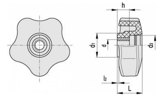
$\begin{array}{lll} D & = 50 \\ \text{d1} & = 19 \\ \text{d3} & = 15.5 \\ \text{dh} & = 8 \\ \text{h} & = 10 \\ \text{I2} & = 1.2 \\ \text{L} & = 20 \\ \text{Weight in (g)} = 23 \end{array}$
